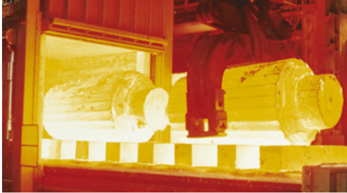
Metallurgical industry: forging furnace
