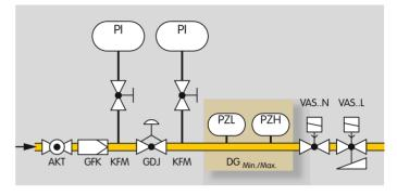
If the pressure is either too low or too high, the min./ max. pressure switch DG (PZL/PZH) switches in order to avoid start-up or to initiate a safety shut-down.
