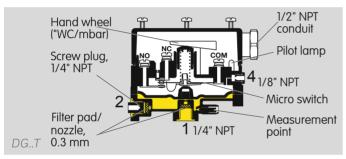
The pressure switch DG switches in the event of increasing or decreasing pressure. Once the set switching point is reached, a micro switch is activated in the DG which is designed as a change-over contact.
